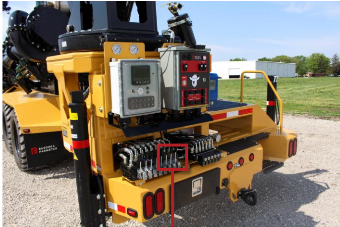
Agitation valve controller location
