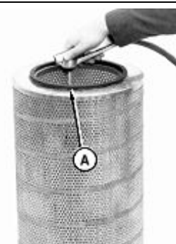
Cleaning Primary Element
