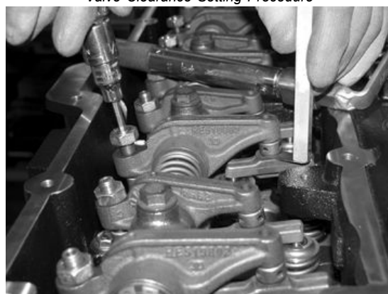
Checking Valve Clearance Using Bent Feeler Gauge
